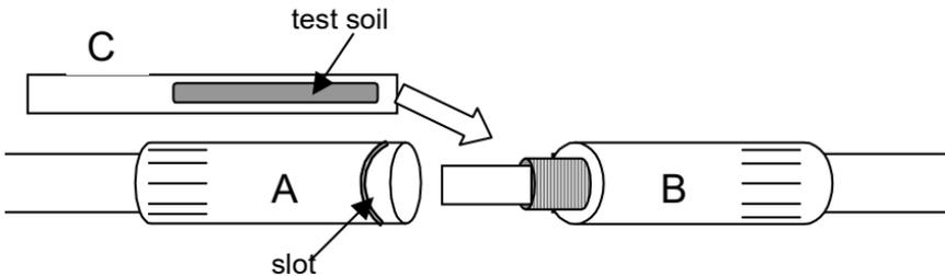
1. Unscrew LumCheck-device: detach part A (marked with slot) from part B (see picture).
